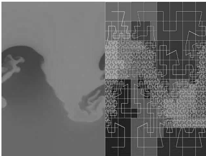
Figure 1. Simulation of a Rayleigh-Taylor instability. Load balancing is based on a Hilbert curve distribution (right side)
