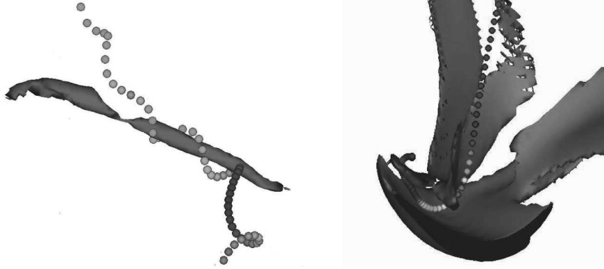
Figure 6. Particle trajectories near singular events (left: Navier-Stokes, right: MHD)
